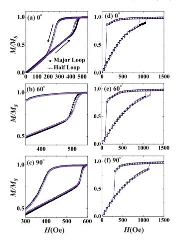
FIG. 2. (Color online) (Left) Measured major and half loops using MOKE, and (Right) simulated major and half loops with the applied field at  $(a, d) \ 0^{\circ}$ ,  $(b, e) \ 60^{\circ}$ , and  $(c, f) \ 90^{\circ}$  relative to the flat edge of the dots.
