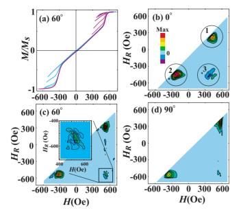
FIG. 3. (Color online) (a) Measured FORC's and (b–d) FORC distributions with the applied field at (b) 0°, (a) and (c) 60°, and (d) 90° relative to the flat edge of the dots. Circles in (b) highlight the three regions of FORC features. Inset in (c) shows a zoom-in view of the negative-positive-negative set of features.
