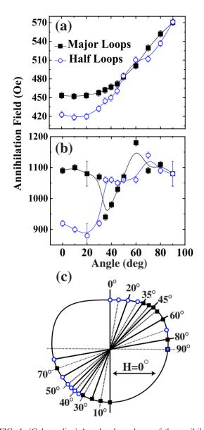
FIG. 4. (Color online) Angular dependence of the annihilation fields from both major (solid squares) and half loops (open circles) extracted from (a) MOKE measurements and (b) micromagnetic simulations. Error bars are included to indicate the field spacing of the measurements and the lines are guides to the eye. The locations of the simulated vortex core annihilation sites are shown in (c). Lines are used to highlight the annihilation sites for each angular position.
